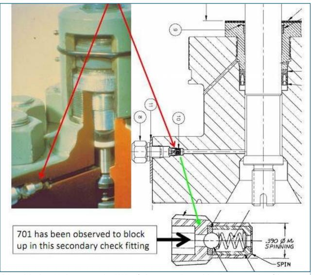
Prior to injecting 701, the operator should identify the exact make, model and pressure rating of the gate valve, and confirm the arrangement of the sealant injection fitting (s) in the valves bonnet. If there is any doubt, it is recommended that test pumping 701 through a spare fitting, attached to the pump delivery hose end should be conducted before injection into the valve.
